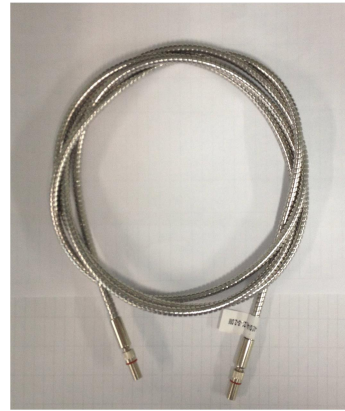
Wrong tie up method
