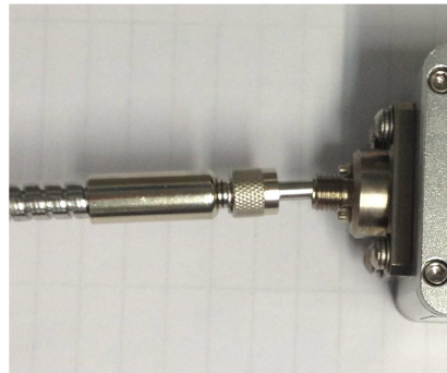
Wrong connection mode
